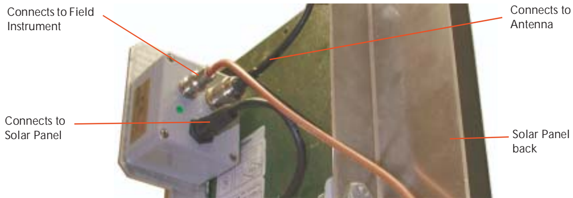
Figure 22 Bias Tee on Solar Panel (applies to cellular Field Instruments only).
